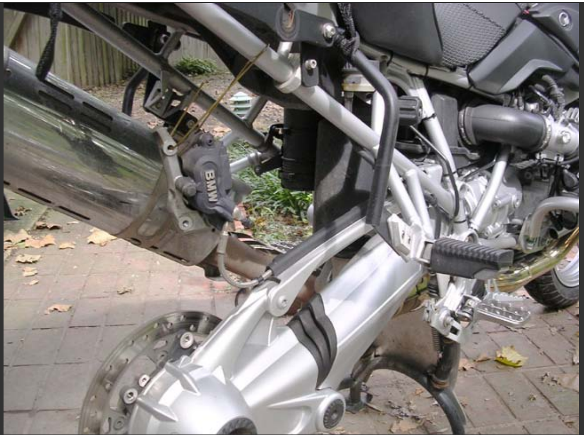
3. Unbolt the Brake Caliper (T-45 Torx) and hang it with some wire to the frame.
