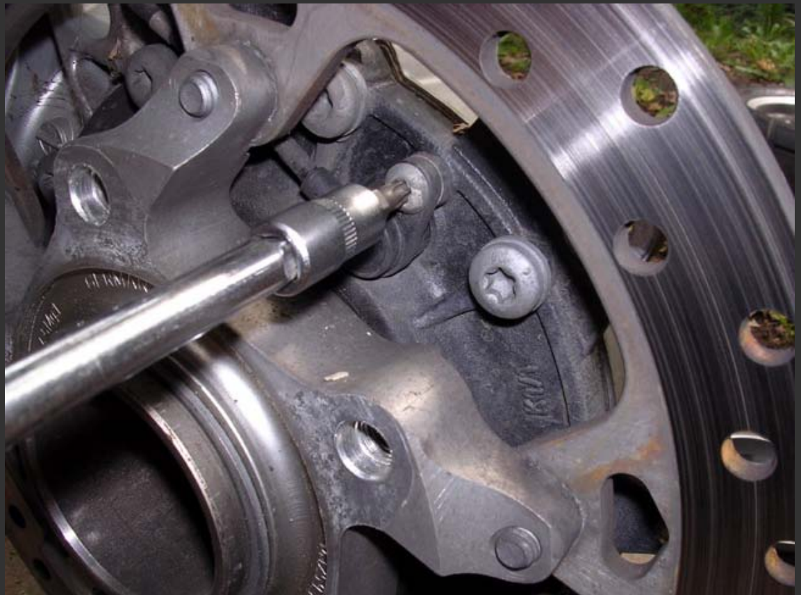
3. Unbolt the Brake Caliper (T-45 Torx) and hang it with some wire to the frame.
